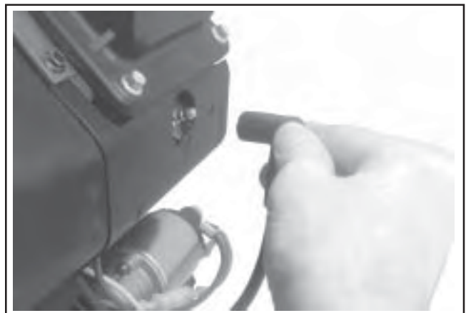
Figure 9-1. Disconnect Both Spark Plug Leads.
