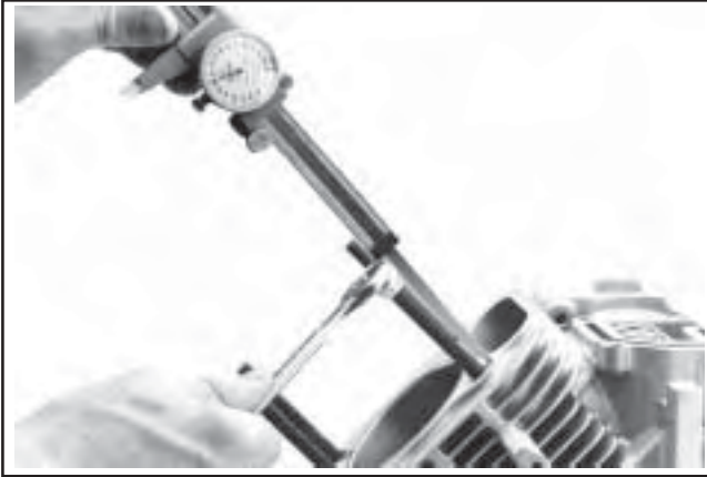
Figure 11-43. Installing New Mounting Studs to Specified Height.
