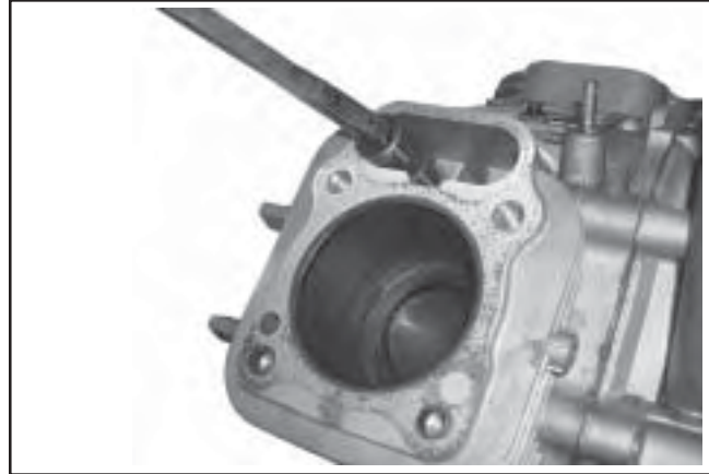
Figure 9-53. Removing Hydraulic Lifter.
