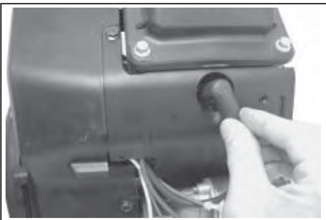
Figure 11-106. Connect Spark Plug Leads.
