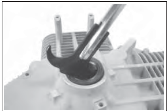
Figure 9-77. Removing Oil Seal.
