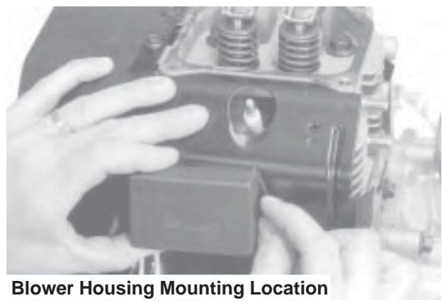
Figure 11-72. Reinstalling SAM Module.
