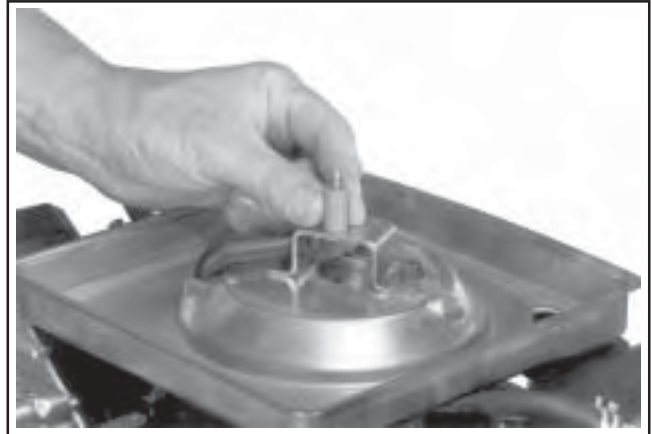
Figure 9-8. Removing Air Cleaner Base Retainer.
