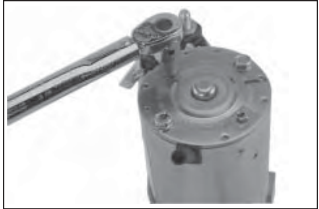
Figure 8-72. Torquing Brush Holder Screws.
