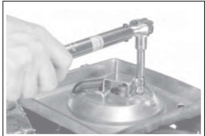
Figure 11-94. Torquing Base Screws.
