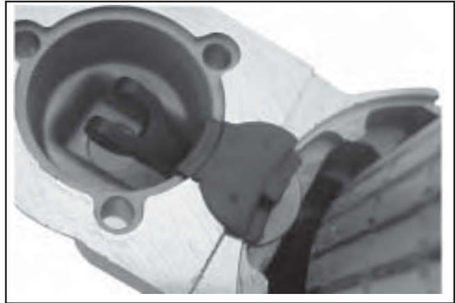
Figure 8-64. Installing Backup Washer and Grommet.
