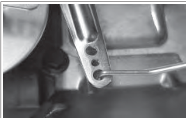
Figure 5B-40. Throttle Link in Center of Hole.
