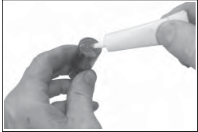
Figure 11-34. Applying Camshaft Lubricant to Bottom of Lifters.
