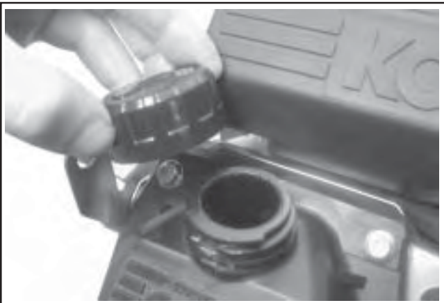
Figure 9-3. Removing Oil Fill Cap from Cover.
