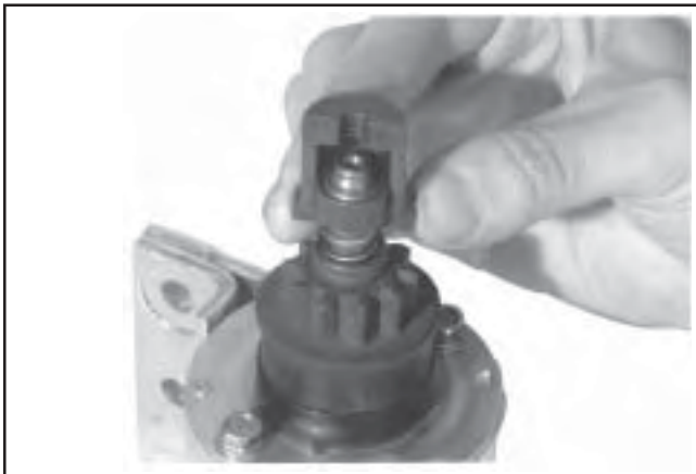
Figure 8-38. Assembling Larger Inner Half Around Spring Retainer.
