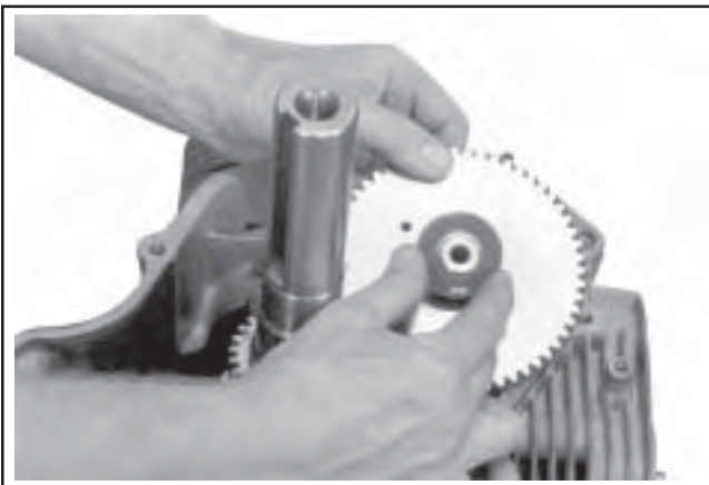
Figure 11-15. Change Shim to Obtain Correct End Play.
