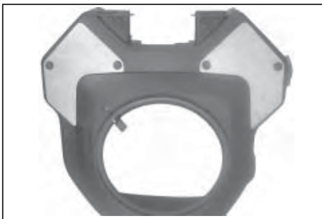
Figure 4-15. Cleanout Kit Installed on Blower Housing.
