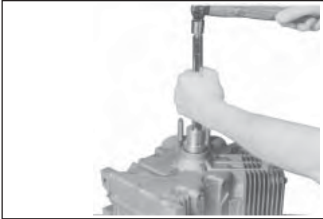
Figure 11-2. Installing Oil Seal.
