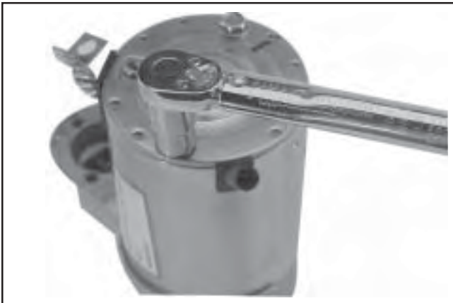
Figure 8-71. Torquing Thru Bolts.
