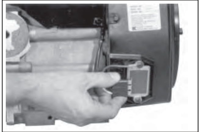
Figure 9-31. Disconnecting Plug from Rectifier-Regulator.
