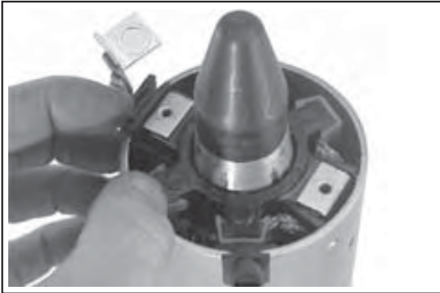
Figure 8-70. Installing Brush Holder Assembly using Tool with Extension.
