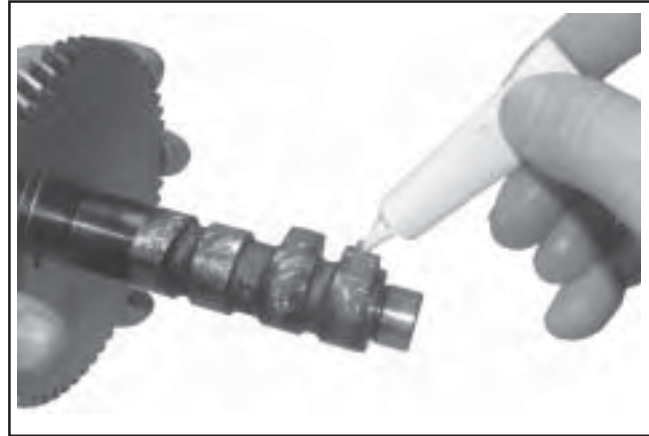
Figure 11-12. Apply Camshaft Lubricant to Cam Lobes.
