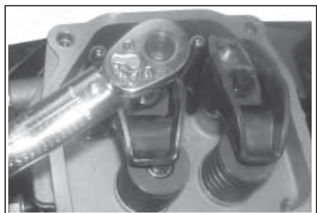
Figure 11-46. Torquing Rocker Arm Screws.
