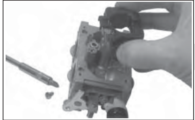
Figure 5-23. Removing Float and Inlet Needle.
