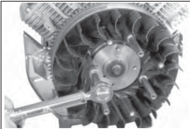
Figure 11-33. Torquing Supports for Metal Screen (Some Models).
