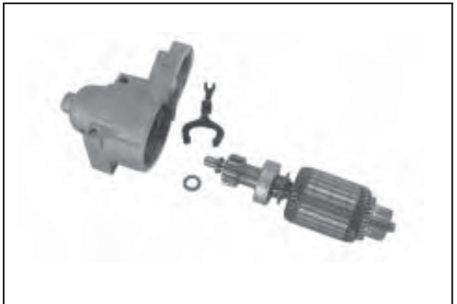
Figure 8-52. Armature and Lever Removed.
