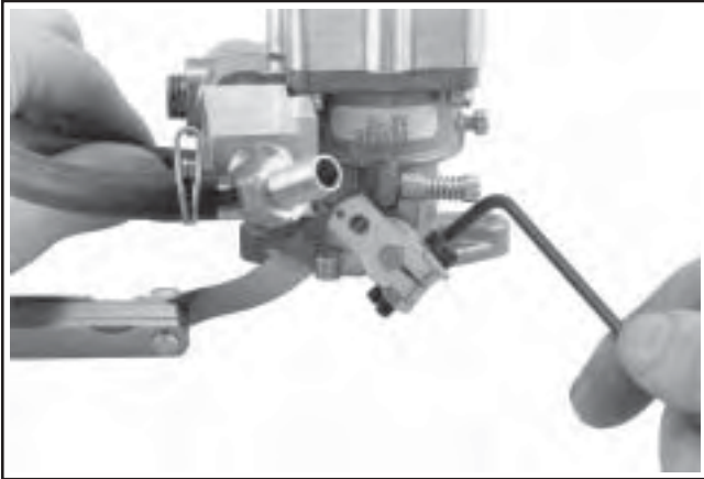
Figure 5A-10. Tightening Idle Speed Clamp Mounting Screw.
