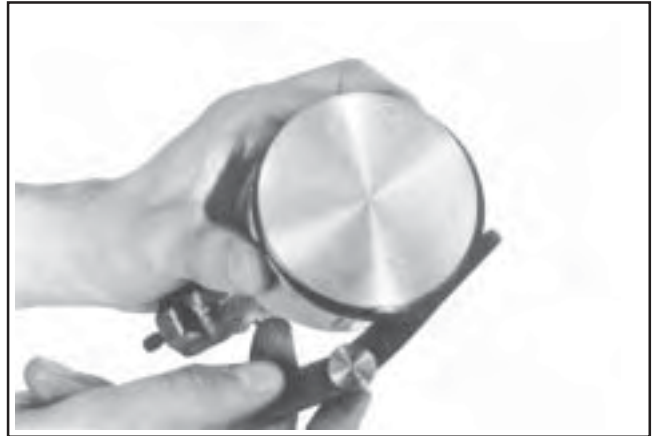
Figure 10-10. Measuring Piston Ring Side Clearance.
