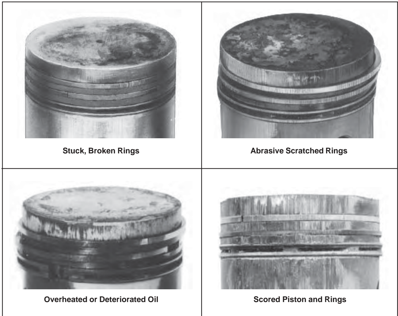
Figure 10-8. Common Types of Piston Damage.
