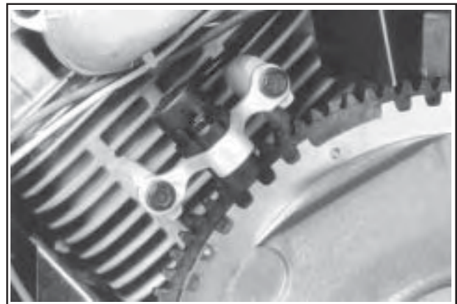
Figure 5B-4. Engine Speed Sensor.
