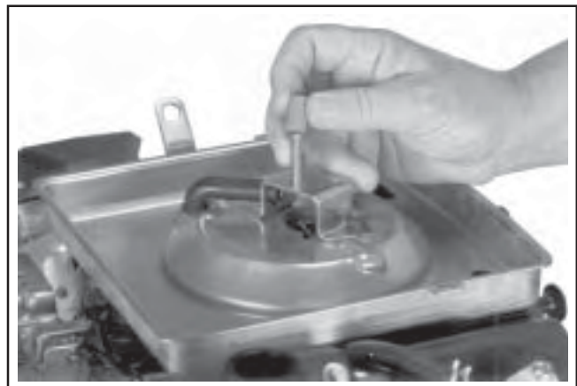
Figure 4-7. Removing Rubber Seal from Bracket.
