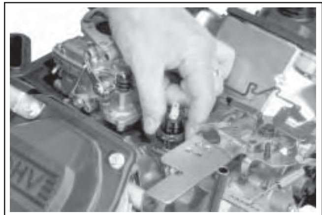
Figure 11-88. Installing Oil Sentry™ Switch.
