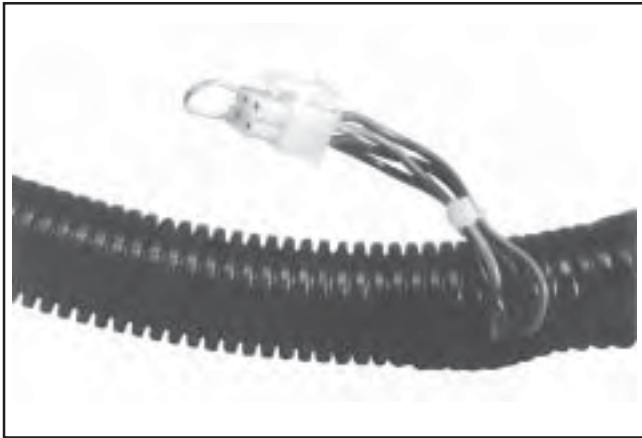
Figure 5B-8. Service Connector Plug, Metal-Cased ECU Harness.
