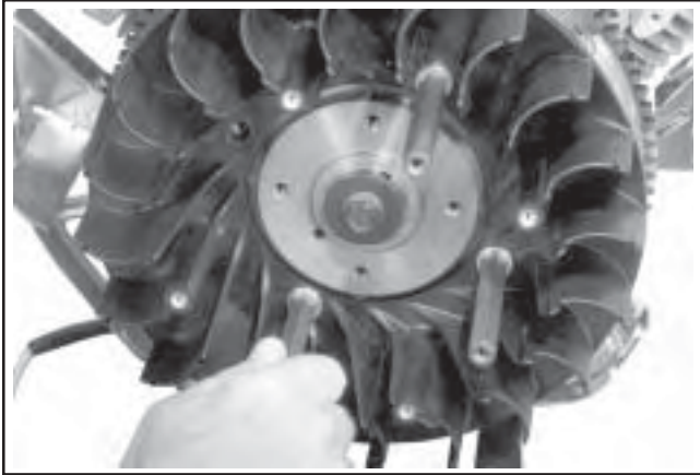
Figure 11-32. Installing Supports for Metal Grass Screen.
