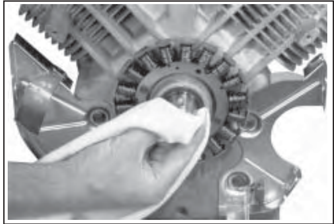
Figure 11-26. Clean and Dry Taper of Crankshaft.
