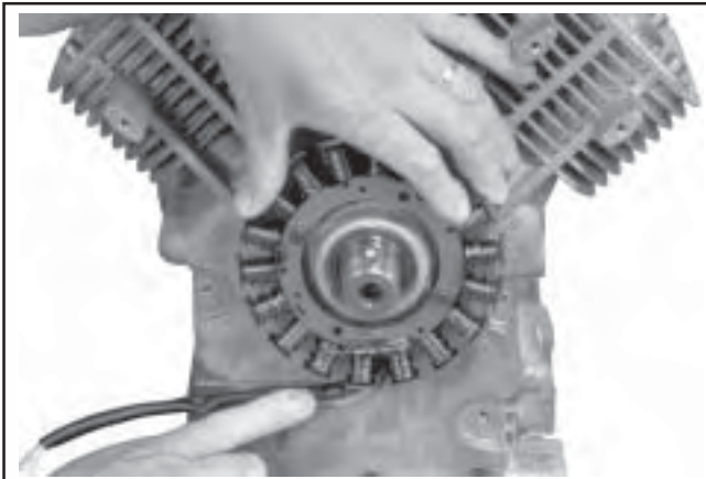
Figure 11-24. Route Stator Leads in Groove.
