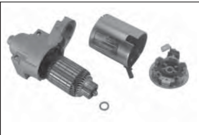
Figure 8-50. Starter Frame Removed.
