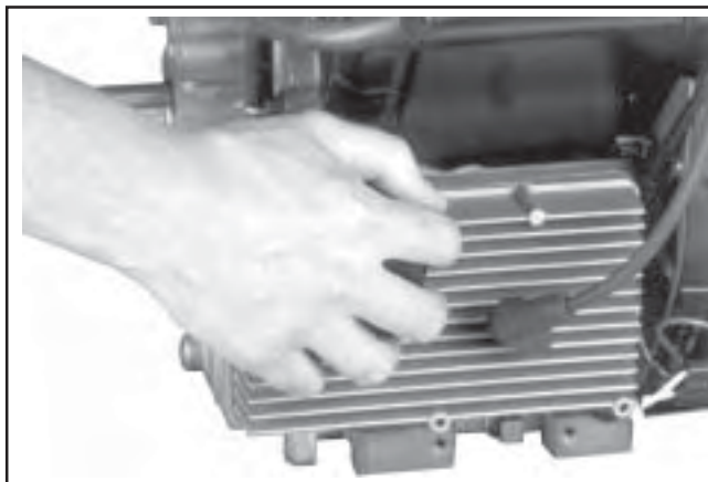
Figure 11-102. Hand Tightening Oil Filter.
