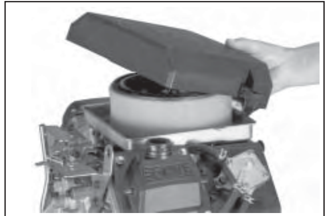
Figure 4-2. Removing Latch Style Cover.
