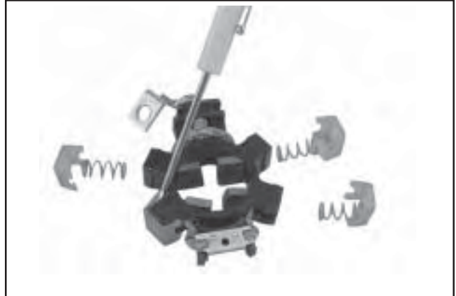
Figure 8-68. Removing Retaining Clips.
