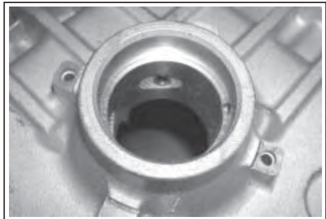
Figure 11-1. Seal Bore of Crankcase.
