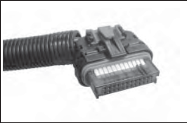
Figure 5B-24. “24 Pin” (MSE 1.0) Plastic-Cased ECU Connector.
