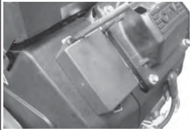
Figure 9-33. Removing the Spark Advance Module (Applicable Models).
