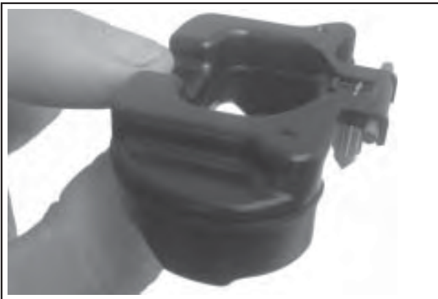
Figure 5-29. Float and Inlet Needle Details.
