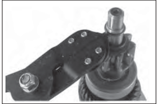
Figure 8-54. Removing Retaining Ring.
