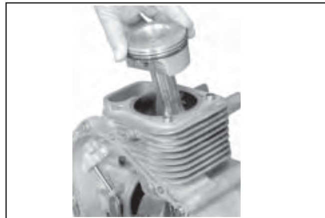
Figure 9-72. Removing Piston/Connecting Rod Assemblies.
