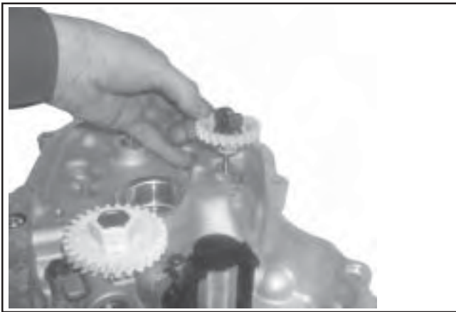
Figure 10-13. Removing Governor Gear.
