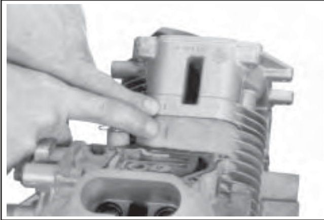
Figure 11-36. Match Numbers on Cylinder Barrel and Head.
