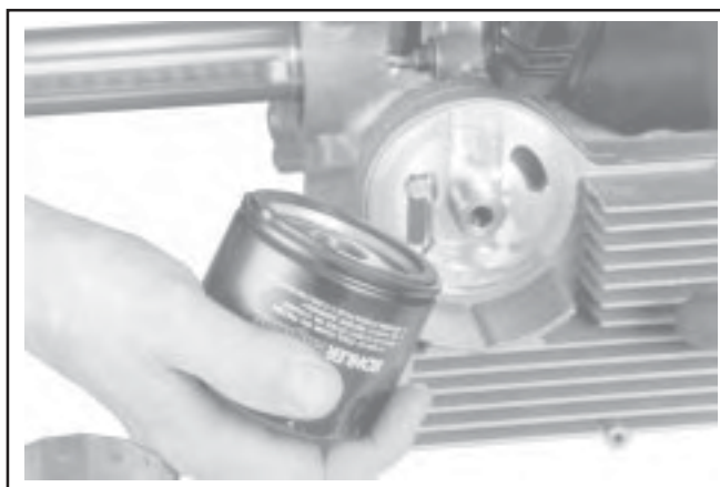
Figure 11-101. Installing New Oil Filter.
