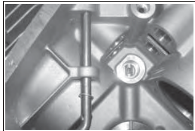
Figure 11-5. Installing 8 mm Governor Cross Shaft.
