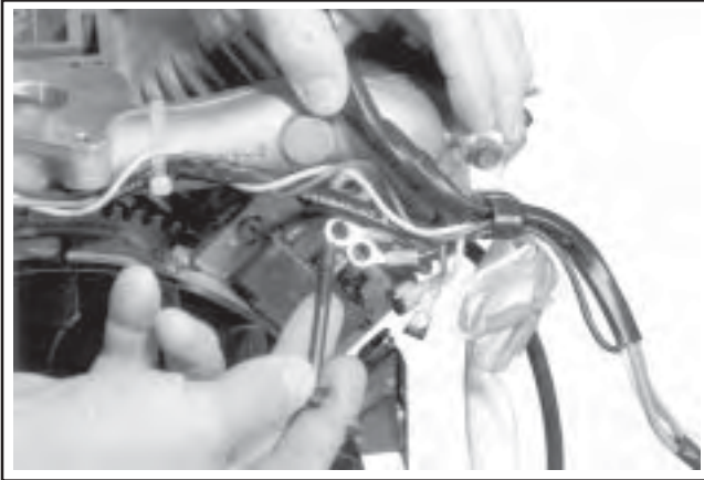
Figure 9-49. Bolt Wiring Harness Detail.
