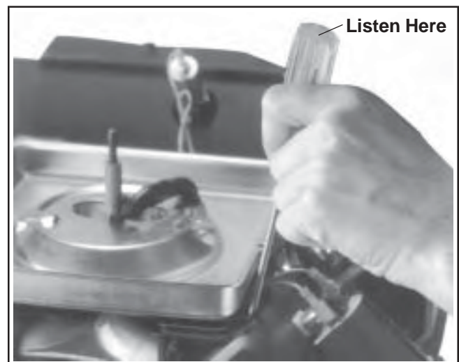
Figure 5B-19. Checking Injectors.
