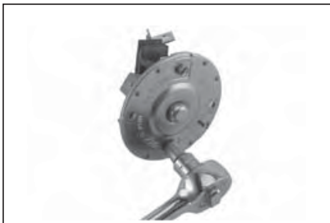
Figure 8-59. Removing Brush Holder.
