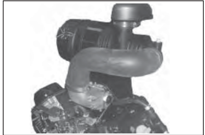
Figure 11-98. Assembled Heavy Duty Air Cleaner (Two-Barrel Carburetor).
