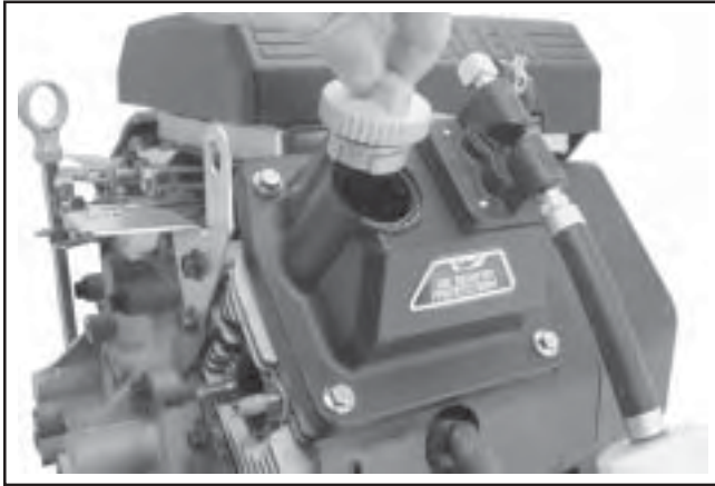
Figure 6-5. Removing Oil Fill Cap.
