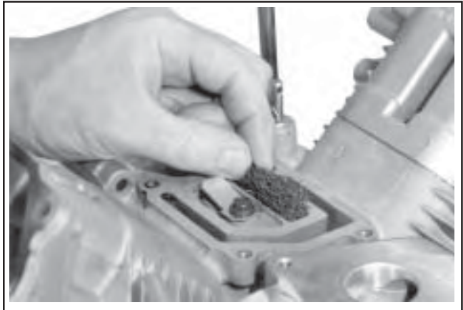
Figure 11-57. Installing New Breather Filter.
