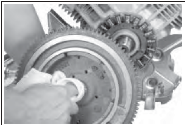
Figure 11-27. Clean and Dry Flywheel Hub.
