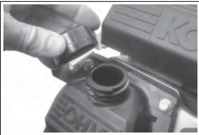
Figure 11-105. Reinstalling Oil Fill Cap (Some Models).
