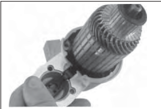
Figure 8-63. Installing Armature and Pivot Lever.
