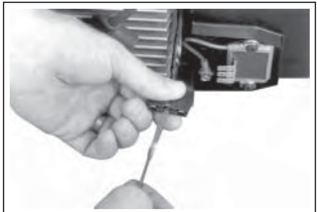
Figure 9-32. Remove B+ Lead from Terminal Plug.
