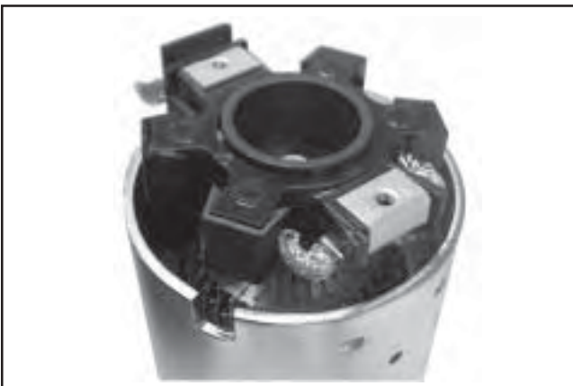
Figure 8-67. Installing Brush Holder Assembly with Supplied Tube.
