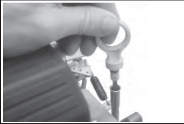
Figure 11-104. Reinstall the Dipstick in Tube.
