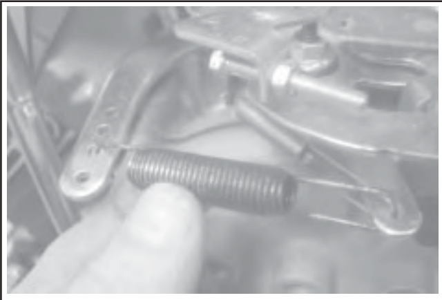
Figure 11-85. Connecting Spring to Governor Lever.
