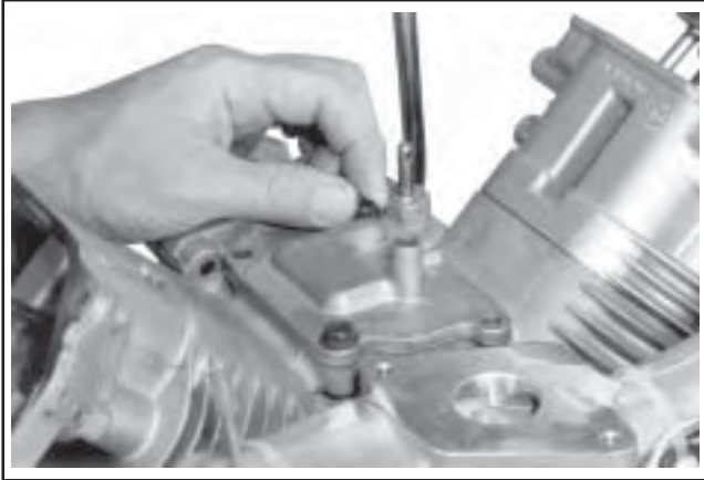
Figure 11-58. Installing Screws (Locations 3 and 4).
