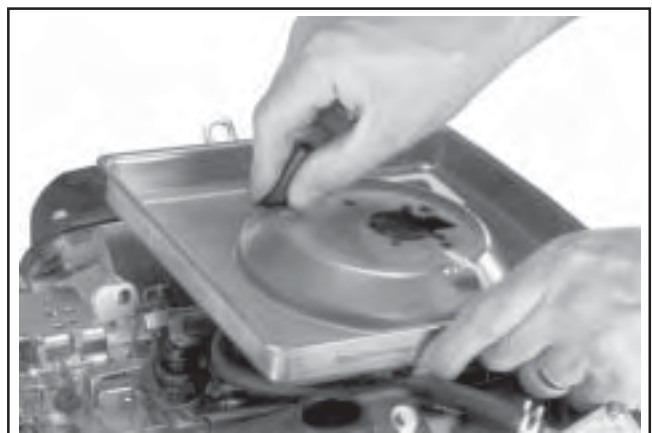
Figure 9-10. Removing Breather Tube from Base.
