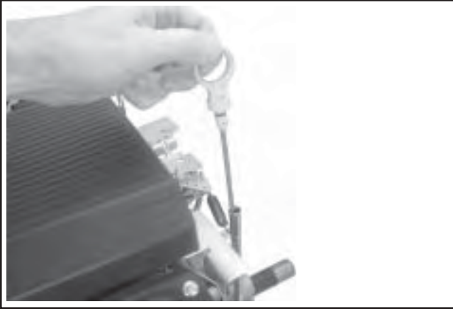
Figure 9-2. Removing Dipstick from Tube.
