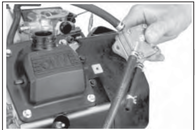
Figure 9-19. Remove Fuel Pump and Lines.
