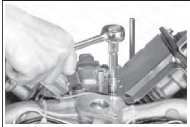
Figure 9-39. Removing Fasteners Holding Baffle and Breather Cover.
