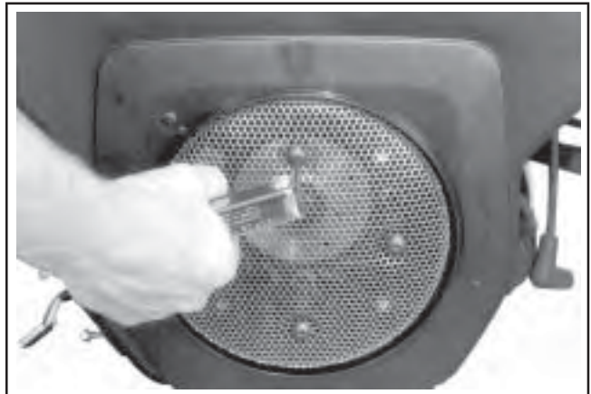
Figure 9-36. Removing Metal Grass Screen.
