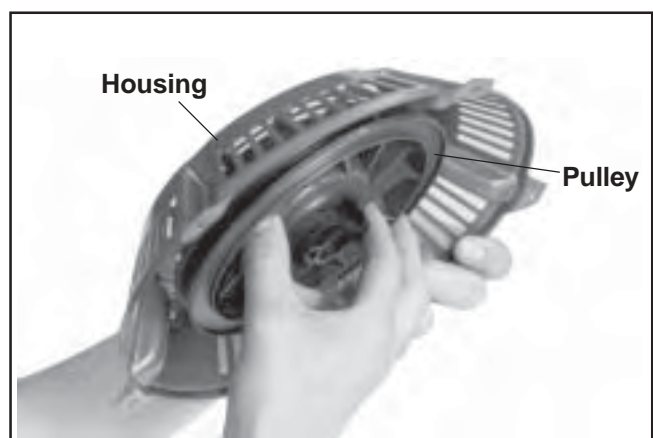
Figure 7-6. Removing Pulley from Housing.
