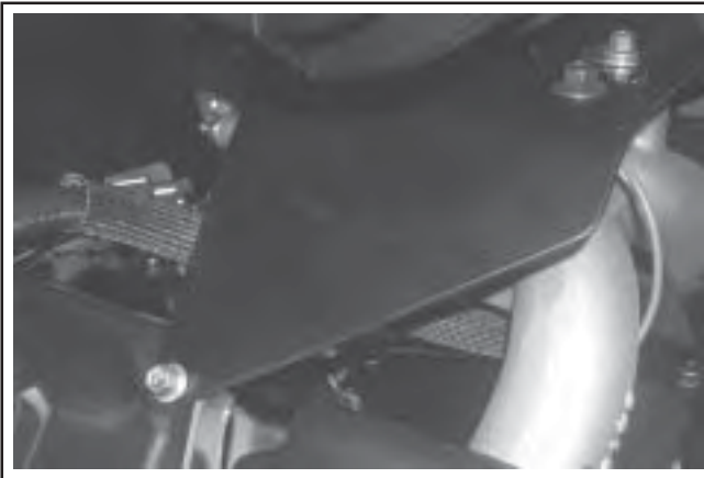
Figure 11-97. Mounted Air Cleaner Bracket (Two-Barrel Carburetor).
