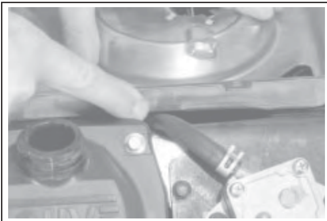
Figure 11-93. Fuel Inlet Line Detail.
