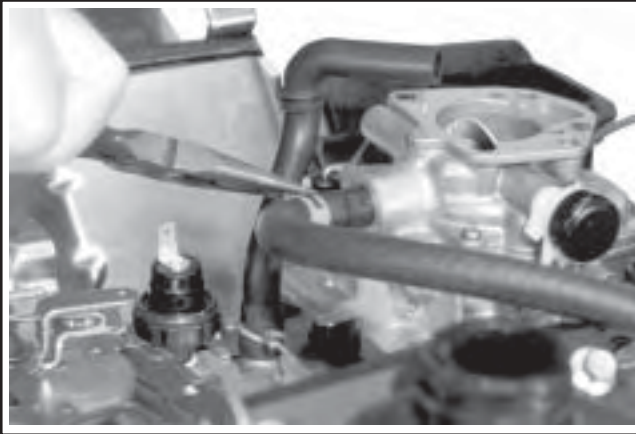
Figure 9-15. Disconnecting Fuel Inlet Line at Carburetor.
