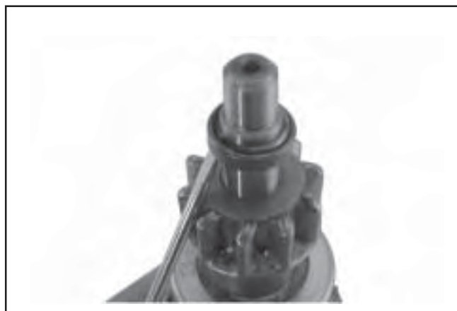
Figure 8-61. Installing Stop Collar and Retainer.
