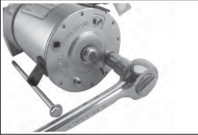
Figure 8-48. Removing Thru Bolts.
