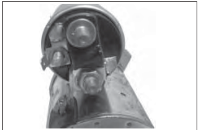
Figure 8-73. Positive (+) Brush Lead Connection.
