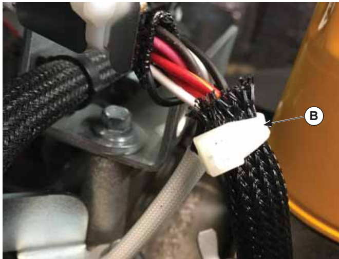
B Cut Wire Tie to Access Spade or Butt Connector
